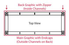
6. Install the fabric graphics. See graphic installation instructions for details. It is most common for the front graphic to start on the back, wrap around the left side, front, right side, and end on the back. 7. Unfold and rest the countertop on top.
