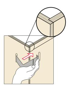
3. Attach clip so that the long leg spans across the edge of the overlapping board. Then, push the knee of the clip until it snaps into the slot.
