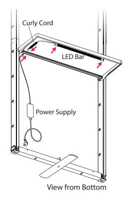
3. Install the optional LED bar to the bottom of the shelf. The bar snaps into the channel in the front, underside of the shelf. The curly cord connects to the power supply cord through the hole in the back edge of the shelf.
