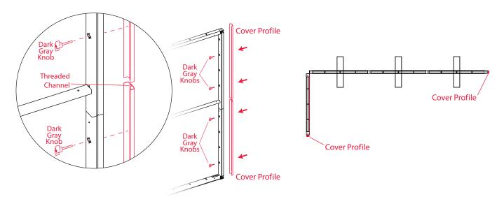
9. To cover the slots at the end of the frames, attach cover profiles with dark gray knobs as seen above. The knobs attach to the cover profile's threaded channel.
