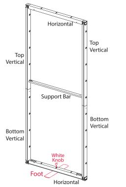
4. Repeat steps 1-3 to build a second frame. 5. Attach a foot to the frame and secure with a white knob.
