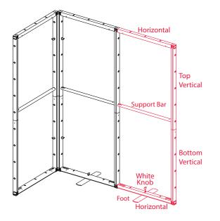
7. Extend the backwall by adding two more horizontals, foot with white knob, bottom vertical, top vertical, and support bar as seen above.
