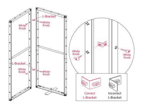
6. Connect the two frames together witht two standard L-brackets and four white knobs. This forms the back/left corner of the display.
