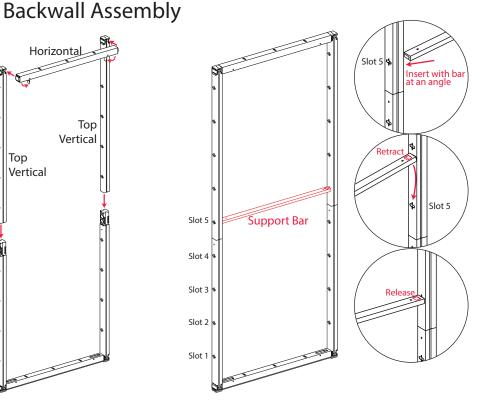
1. Assemble the first frame by connecting one horizontal bar between two bottom verticals, lift the lock levers, slide the parts together, and close the lock levers.
