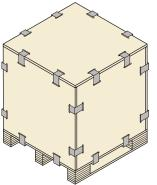
8. Be sure the top is fully seated, then attach with the remaining clips.
