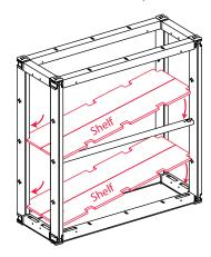
5. Unfold and rest one shelf on the bottom horizontal bars. Unfold and rest the second shelf on the support bars.
