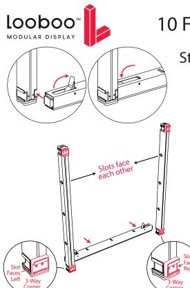
1. Locate two short vertical bars with 3-way corners on both ends. Attach the two together with a horizontal bar by lifting the lock levers and sliding the parts together.
