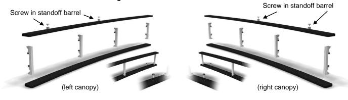
Step 4. Insert plex w/ pre-installed puck lights. Attach one 3-way power splitter to left 3 lights and one to right 3 lights.
