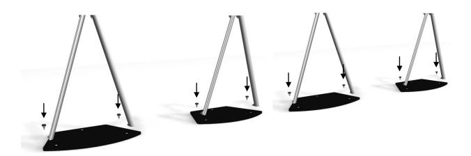
Step 12. Attach V-leg counters to backwall & bases using 3 long knobs per counter.
