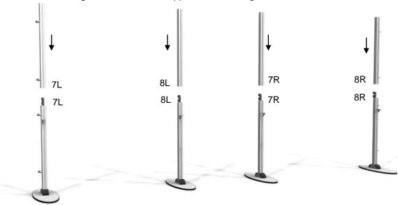
**Step 9**. Connect upper and lower graphic hangers. Slide upper and lower graphic hangers into graphic and hang graphic.
