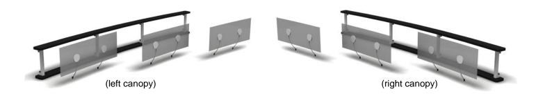
Steps 5&6. Attach left and right lower columns to feet using 2 short thumb knobs per column. Install gusset caps.
