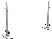
**Steps 7&8**. Attach left and right lower columns to upper columns using 2 **short** knobs.
