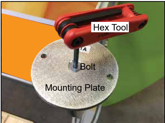
5) Tighten bolt, using hex tool, to secure.
