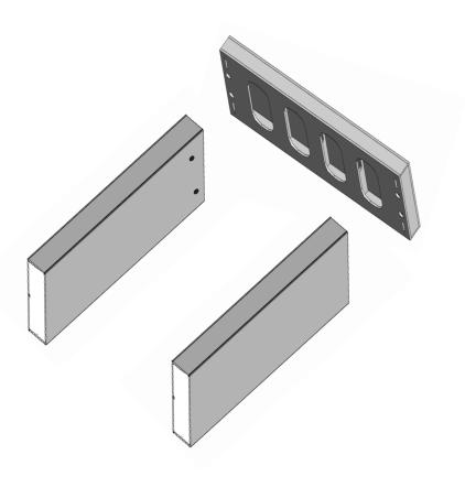
2. Push the side panels into the top panel and engage the roto locks with the hex key. Tilt the counter upright to complete the assembly.
