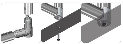
Take the plastic connector and make sure the snap buttons are in proper position for the frame tube holes. Simply press the snap button with your thumb and carefully slide the tube onto the connector. The snap button should pop through. Some twisting may be necessary to assure the snap button has popped all the way through the tube hole. Do not force the connection and be careful with the tube edges, they may be sharp.
