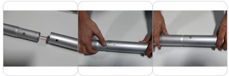
For snap button connections, locate the snap button on the connector or swage tube. Locate the hole on the corresponding tube. Press the snap button with your thumb and slide the tube and connector together so that the snap button snaps fully into the lock hole. To disassemble, press the snap button and pull apart.
