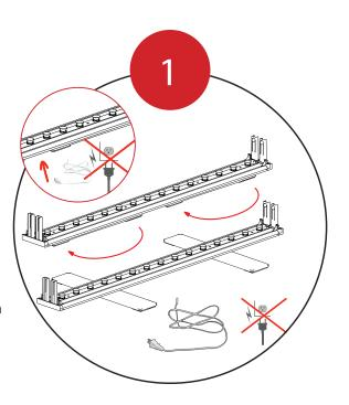
Fit the Side Extrusion Bottoms onto the Bottom Extrusion connectors.
