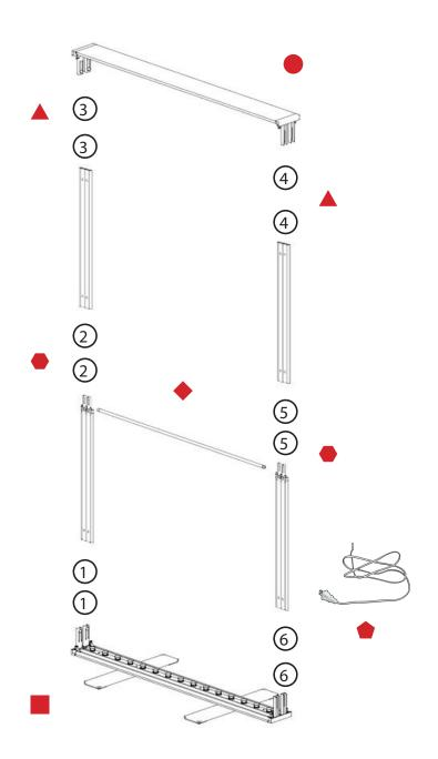
Swivel the feet of the Bottom Extrusion.
