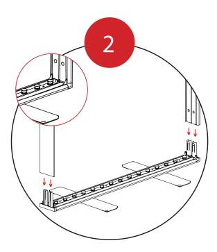
Fit the Side Extrusion Tops ▲ onto the Side Extrusion Bottom ● connectors.
