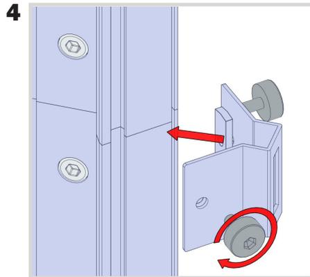
Using the screws provided, attach 8 of the brackets to the joints of your verticals and two at the top of your PMFC2 verticals.
