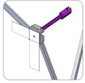
Attach the female arm by popping it into the hub. Fasten the screw through the steel plate hole and the hook and loop fastener webbing tapping into the female arm.
